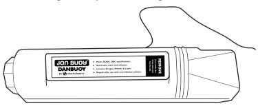
f) Ensure that the 25cm of line is accessible once the container is closed
