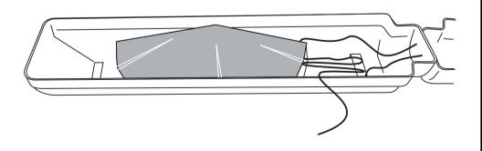
d) Ensure the Lifebuoy attachment loop is towards the centre of the case. Flake the excess lines down the inside of the case, ensuring the Lifebuoy attachment loop is in place throughout. Attach the pouch containing the static line to the cylinder using one turn of electrical tape (25mm wide). Ensure that 25cm of the static line remains outside of the case.
