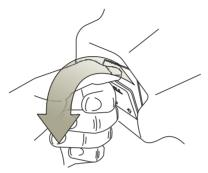
Upon release, the module will Automatically fall outboard and the inflation sequence will be initiated.
